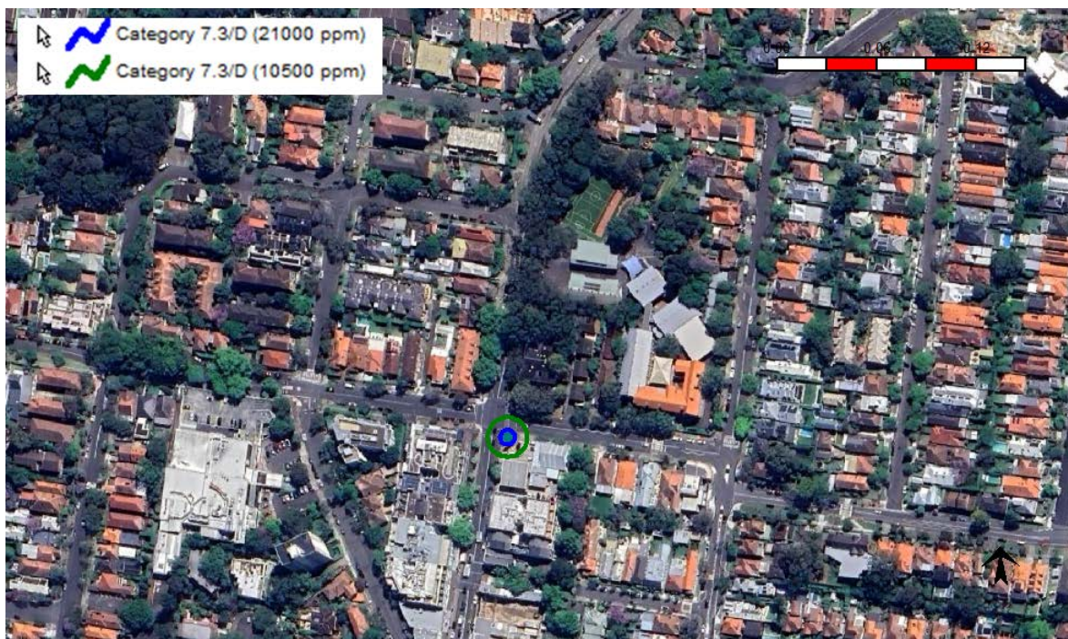
Figure 4: Flash Fire Contours for 8.5 kg Cylinder Rupture (D7.3)
